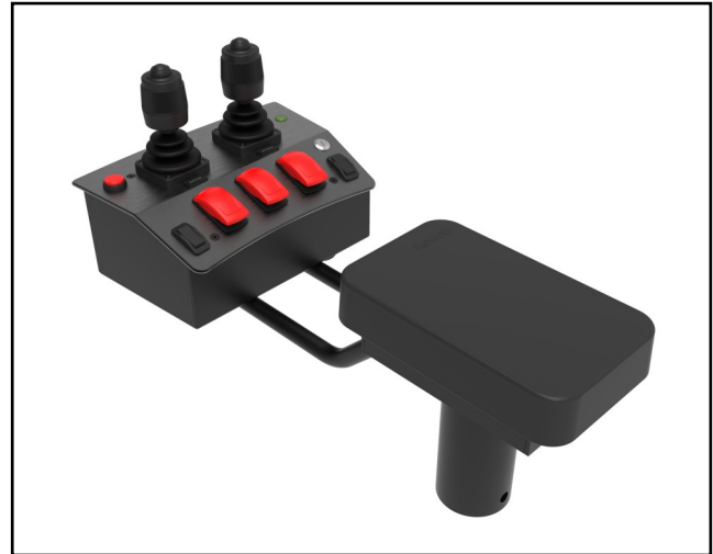
Joystick console series CS-106, with 2 multiple axis joysticks, 3 auxiliary device switches, valve solenoid trim switch and actuator stow mode switch, for the control of multiple functions on plow truck systems. Shown with optional armrest.
