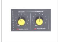
Parameter numbers are selectable by using the spinner and conveyor dials. (For example, setting the spinner dial to 3 and setting the conveyor dial to 5 will show parameter 35 on the screen.)
