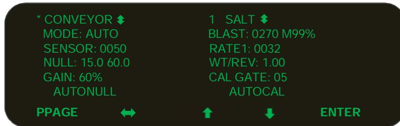
Using **↔** or **↓** move from conveyor configuration to material configuration.
