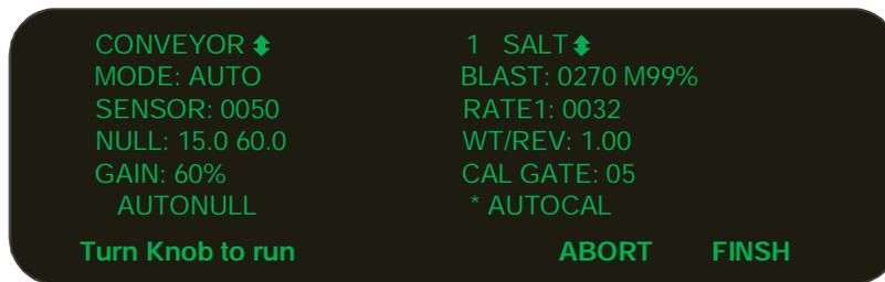
After pressing **FINSH**, the screen will jump to the material weight input screen, enter the weight of the material that was dispensed, the controller will calculate the WT/REV and the result will be displayed on the screen.
