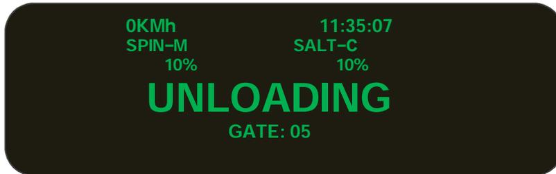
Turn the dials until the desired speed is achieved. Press both the conveyor and the spinner dials simultaneously to exit unload mode. Moving the vehicle will suspend the unload process. It will automatically resume when the truck is stopped again.
