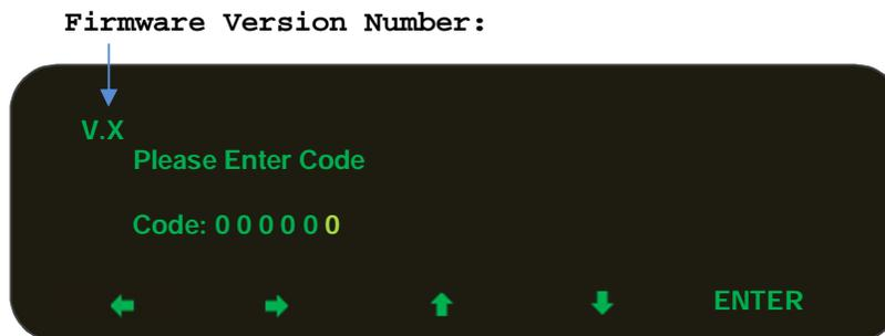
The most right digit stays bright while the rests are dim, pressing the keypads left or right arrows to choose the digit and the up / down arrow to change character (This also applies to the settings of other features). After that, press **ENTER** to confirm the input. The default password is 000000, the user can change this password once in the setup screen.
