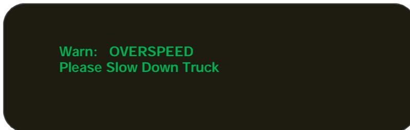
An audible alarm and error message will display on screen for 4 seconds when an error occurs, then it will go off and could come back on 3 minutes later if the error is not resolved. Others more serious errors will stay on the screen until the controller power is cycled or the error is resolved.
