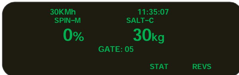
Pressing **STAT** will go to the diagnosis screen which displays the power voltage, actual conveyor RPM and rate.
