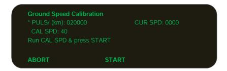
Drive the vehicle and hold the vehicles speed (as indicated on the speedometer) at the value you entered in the CAL SPD field. Press the **START** button.
