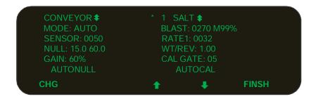
Use up / down arrow to view each material's settings and press **FINSH** to select the material. If **CHG** is pressed, the system will start to edit the material names. (to a maximum of 4 characters)
