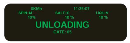
Turn the dials until the desired speed is achieved. Press both the conveyor and the spinner dials simultaneously to exit unload mode. Moving the vehicle will suspend the unload process. It will automatically resume when the truck is stopped again.
