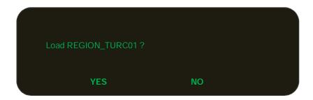
Press YES, the controller will display 'LOADING', when complete touch 'QUIT' and then 'QUIT' again. Touch the 'SETUP' button, then the 'EXIT' button and power the display off. This procedure confirms all the parameters will be refreshed to the controller's memory.
