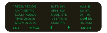
Press up / down arrow to navigate to the different features, the \* symbol preceding the line will mark the active line. Press **ENTER** to edit / select the settings, some fields may also have a sub menu as indicated by the '**CHG'** icon. This is for editing the field. (See example of the editing of REGN below). Press **NPAGE** to go to the next screen and **PPAGE** to the former one.
