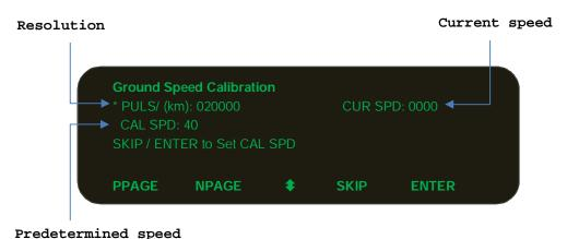
After the predetermined speed is set up, the controller will jump to the following screen and the text message "Run CAL SPD & press START" will flash.
