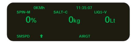
Press the **AIRGT** button to enter the air gate adjustment screen. Press the  $\iff$  button to switch between low gate and high gate. The chosen gate setting is highlighted.
