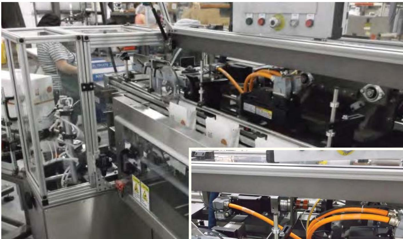
**TOP:** Ultra Packaging's Veronica vertical cartoner provides an efficient, compact cartoning solution that was custom-engineered to handle both conventional and gable-top cartons, using Rexroth's IndraMotion XLC platform for complete automation control and fast changeovers.
