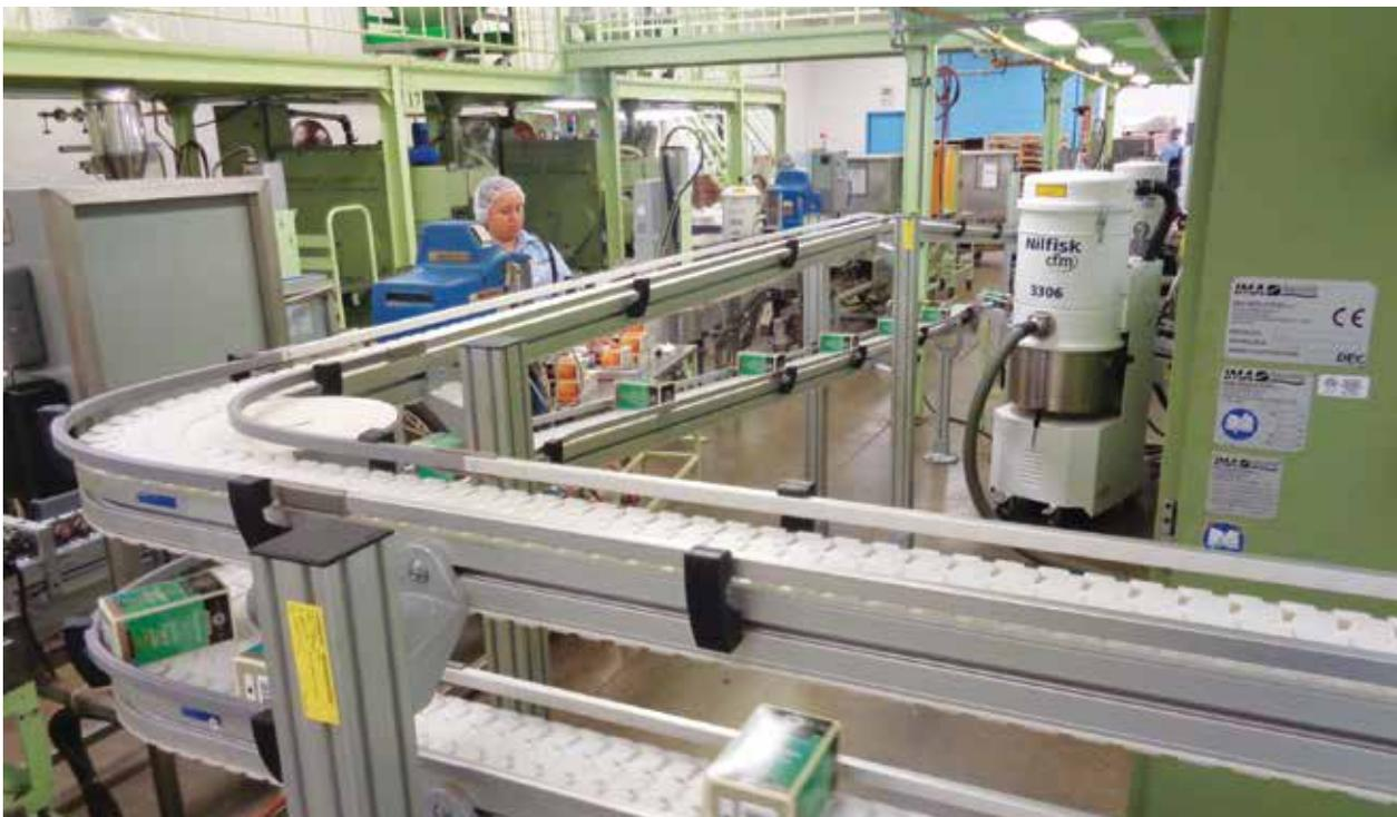
VarioFlow plus' smooth conveyor belt allows the Yamamotoyama to fill shelf-ready cartons that remain neat and unscratched.
