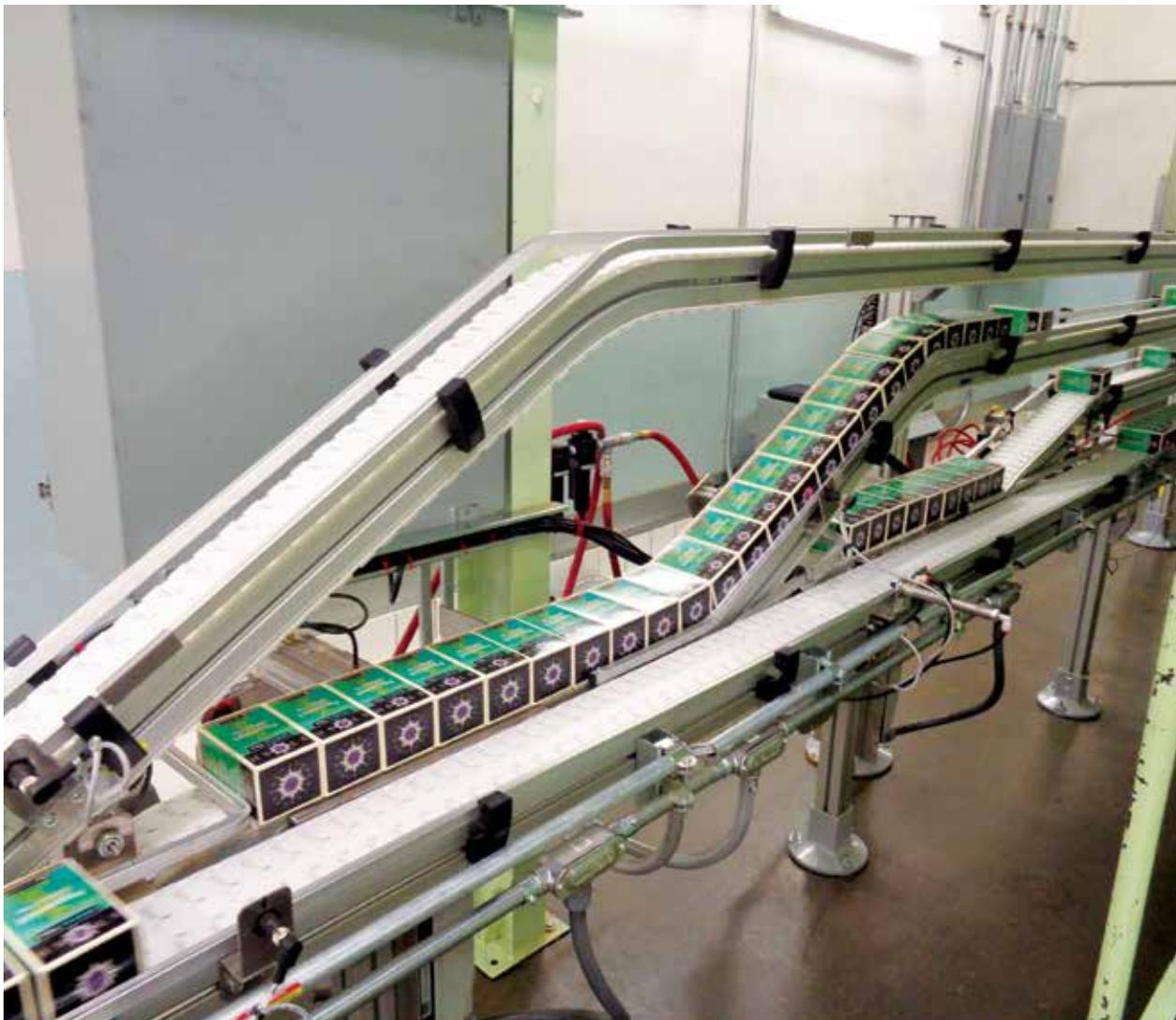
Rexroth's VarioFlow plus allows Yamamotoyama to move products horizontally, vertically, on incline or decline, overhead, sub-floor, around obstacles and over long distances.
